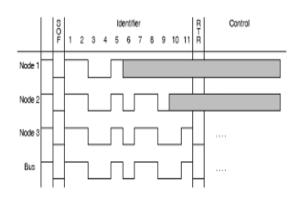
Fig 3(a) Standard CAN Format
